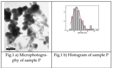
TEM images (Fig.1a) show faced particles with homogeneous size distribution near 23 nm while XRD (inset of Fig.2) confirm spinel phase. Prepared nanoparticles (P) were analyzed by transmission microscopy. TEM images (Fig.1) show faced particles with homogeneous size distribution near 23 nm
