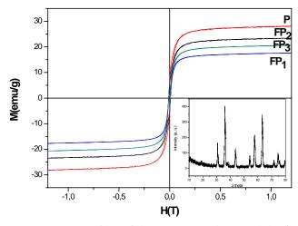
Fig.2. Magnetic profiles of the as prepared (P) and the functionalized (FP<sub>i</sub>) nanoparticles. The inset shows the diffraction pattern of P.
