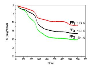
Fig. 4. Thermogravimetric profiles of the functionalized samples
