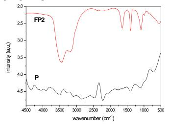
Fig.3. FTIR spectra of magnetic nanoparticles as prepared (P) and one of the functionalized nanoparticles (FP<sub>2</sub>) as example.
